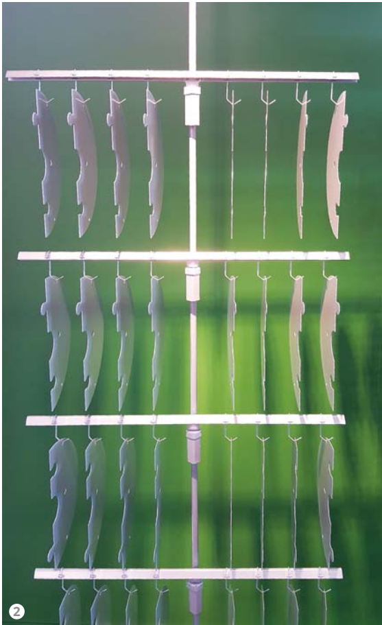
Figure 2: The HQC hanging system, featuring a bar holder with a silicone protection.
